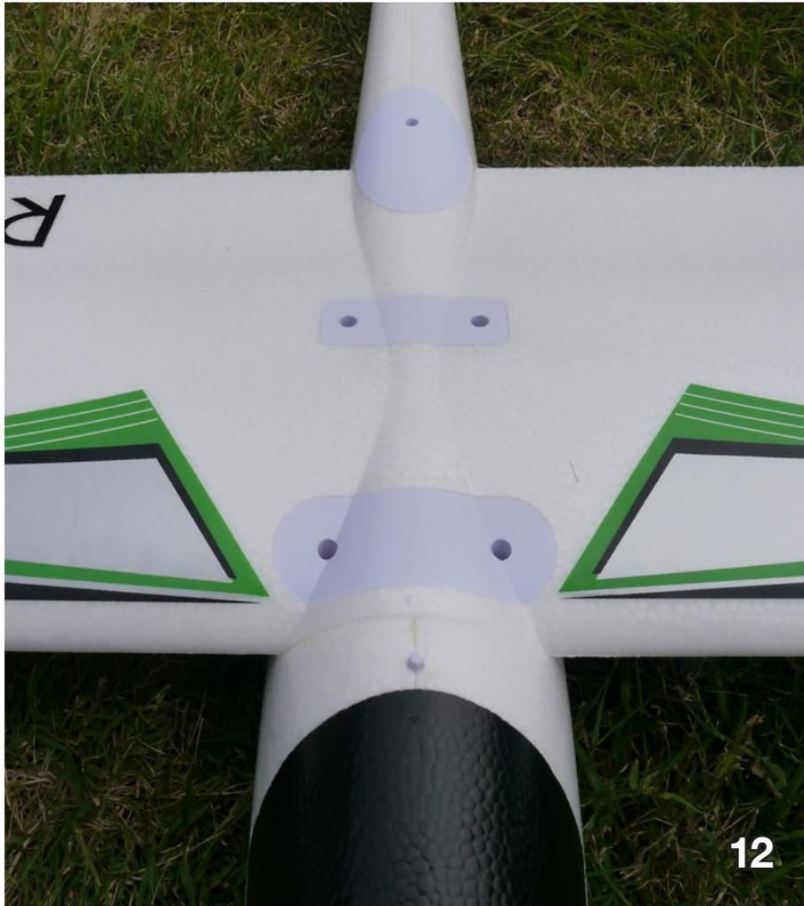
different sizes! You may wish to color-code both the holes and the screws with four different colors of foam-safe paint. And, even though a few extra screws are provided, be sure to do the assembly over a drop cloth: you'll never find the screws in the grass.
