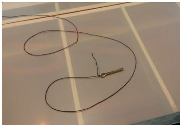
The center panel with the flap servos is a bit more elaborate, since I needed to feed two sets of servo wires through, or at least from the flap servo location inwards.
