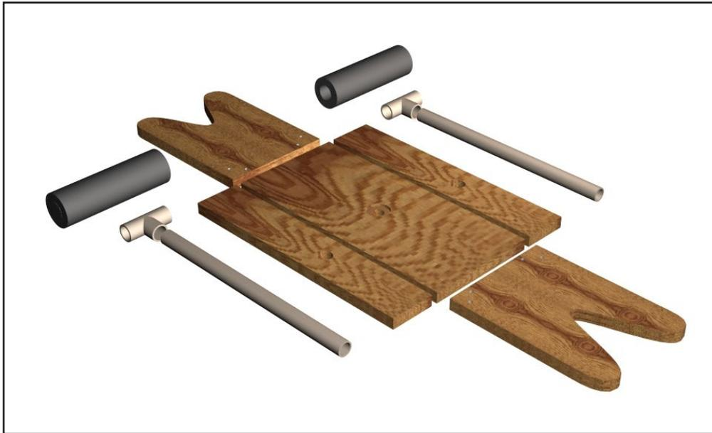
The pan-heads let the side supports adjust and are tightened when you have it positioned where you want it.
