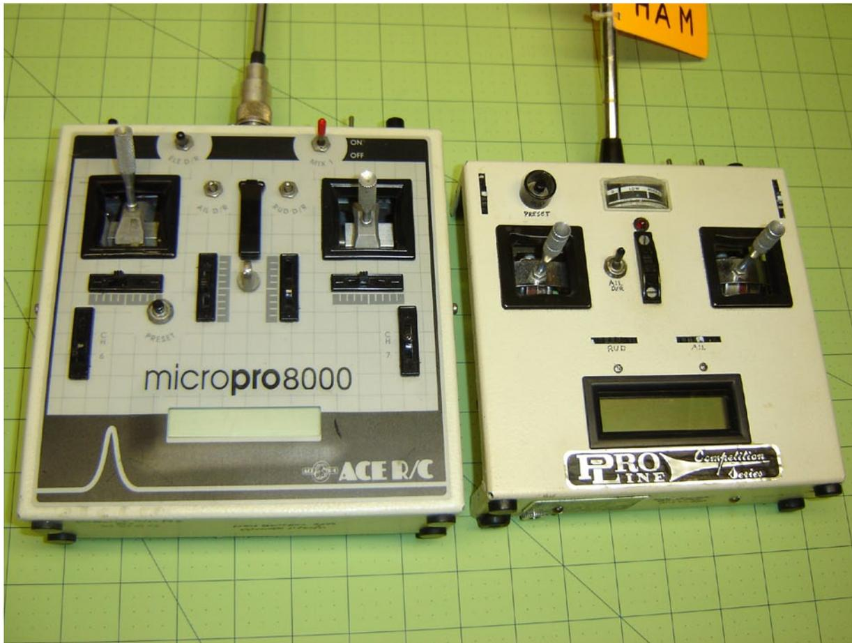
*At left is the original Ace MicroPro 8000 transmitter that started it all. Everything in that case was hand soldered from kits so the larger size was needed. With surface mount technology used on current circuit boards the overall size of the transmitter can be safely downsized.*
