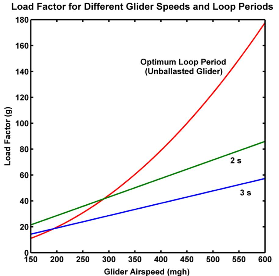
Figure 5. Load factor plotted as a function of glider airspeed and different loop periods for the unballasted glider ( $V_c = 45$  mph). Load factor is equal to the total acceleration of the glider in terms of the acceleration of gravity (g).
