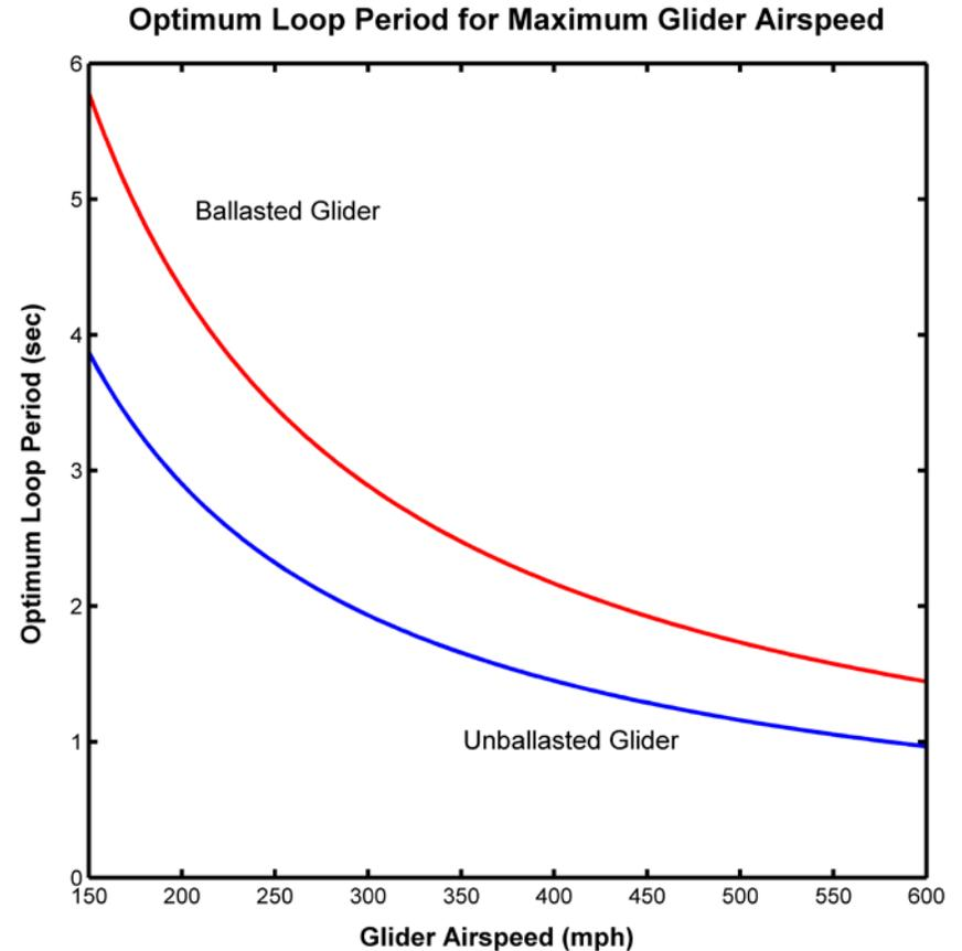
Figure 3. Optimum loop period  $t_{opt}$  required to achieve the maximum glider airspeed in a Rayleigh cycle plotted as a function of glider airspeed. Curves are shown for the unballasted ( $V_c = 45$  mph) and ballasted ( $V_c = 55$  mph) gliders. Ballast is around 50% of the unballasted glider weight.
