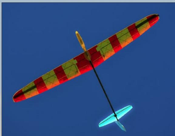
**Front cover:** Phil Pearson captured this image of Ken Lies' DLG at a contest in Pasco Washington last year. Ken built the airframe using a Zone wing. Valspar paints for coloring; red color down first then light layer of yellow over the entire bottom mylar. The tops are solid red which gives the thinner flaperons the orange hue.
