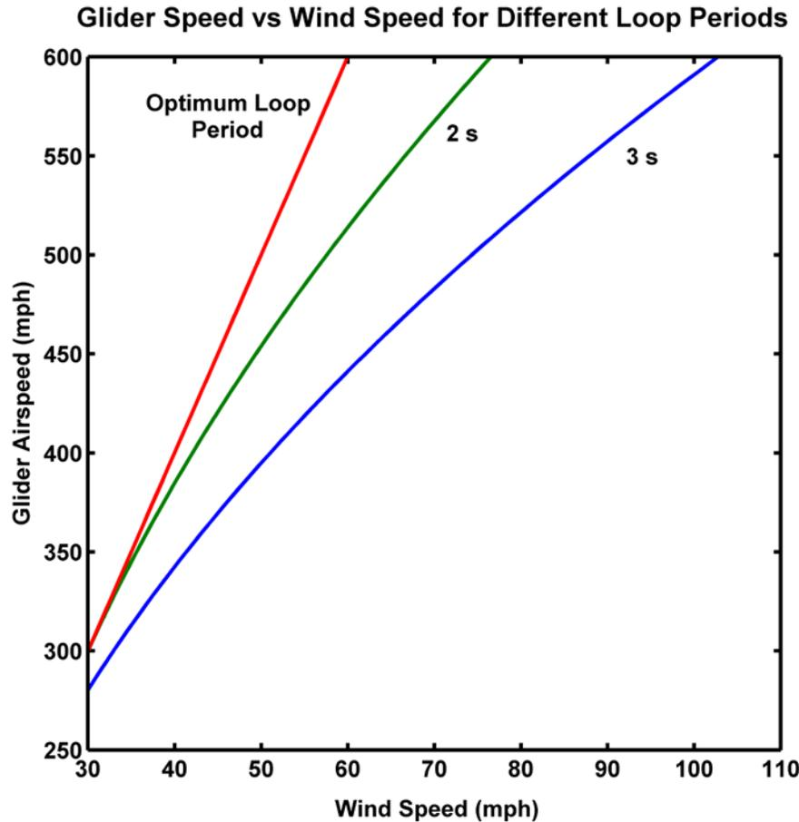
Figure 4. Maximum glider airspeed as a function of wind speed using a Rayleigh cycle and the unballasted glider ( $V_c = 45$  mph). Curves are shown for the (variable) optimum loop period (see Figure 3) as well as for constant loop periods of 2 s and 3 s.
