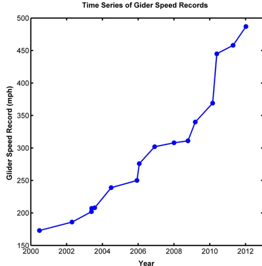
Figure 2. Time series of maximum recorded speeds of RC gliders using dynamic soaring as listed in the website [rcspeeds.com](http://rcspeeds.com). Each value represents an unofficial world record as measured by radar gun. The charted record holder is Spencer Lisenby who flew a Kinetic 100 (100 inch wing span) glider at a speed of 487 mph in January 2012. On 06 March 2012 Spencer flew the Kinetic 100 to a new record speed of 498 mph. <<http://www.rcgroups.com/forums/showthread.php?t=1609281>>
