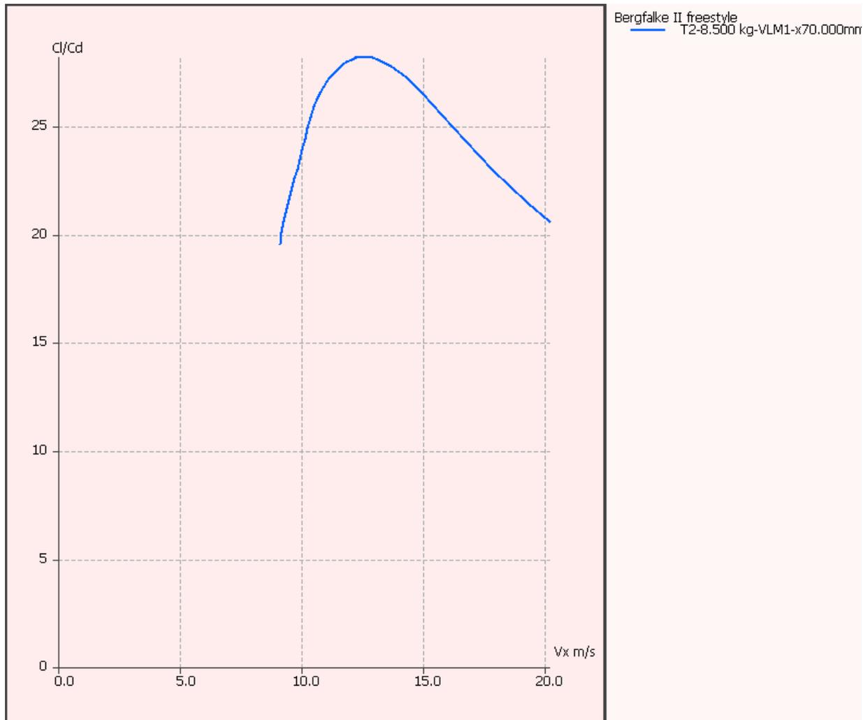
and the model flies balanced at 12.6 m/s with neutral stabilizer trimming.
