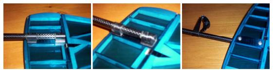
I) Fin may be mounted on either side of boom. Rotational position of fin on boom is not important at this time, unless you want to place the boom mold seam down for appearance. Final fin rotation will be set when boom is glued to the pod.
