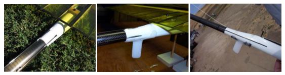
c) Hook up pushrods with your favorite connectors and verify full freedom of movement and adjustability. If using threaded brass connectors, be sure to clean the cavity in which the carbon rod will be epoxied with some alcohol or other solvent/cleaner/degreaser.
