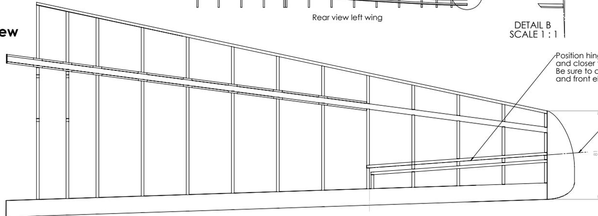
Position hinge axis closer to front elevon spar and closer to the top wing surface. Be sure to close the gap between elevon and front elevon spar.
