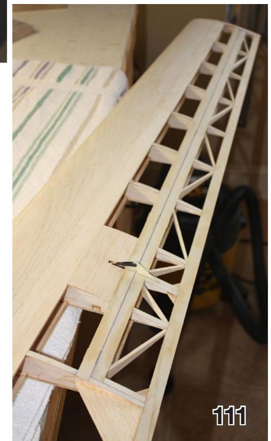
Next bevel the edges of the 1/32" ply on top of the wing and the aileron just about 30 degrees to allow the aileron to move upward 1.5 inch measured at the root end.
