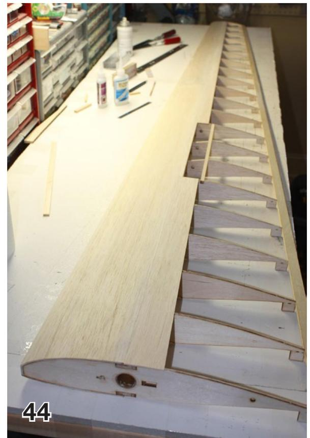
Cut and fit the small 1/32" ply gussets, and the strip of 1/32" ply that goes on top of the 1/4" square basswood, and CA into place. See pix 42 - 44.
