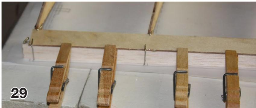
27. All of the trailing edge webs have been sanded. The protective tape is still in place.
