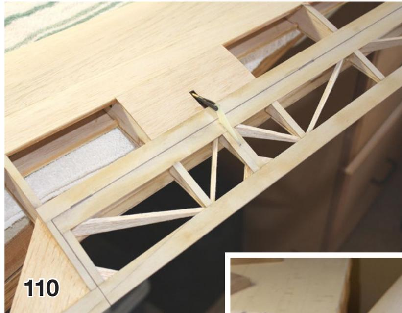
110. Edges of the 1/32" plywood on top of the wing and aileron have been beveled to provide clearance on upward deflection. Here you can see the small gap at the hinge line with the aileron dry fitted.
