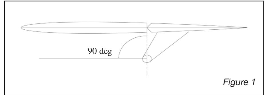
Let's begin by looking at a typical rudder or elevator installation. The pushrod must be connected to the control horn and servo arm at a 90 degree angle from a line between the hinge line and the pushrod attachment point to avoid unequal movement either side of neutral. In the "good old days," we adjusted the angle between the pushrod and aileron horns or control horns to provide aileron differential but that isn't necessary with modern computer radios.
