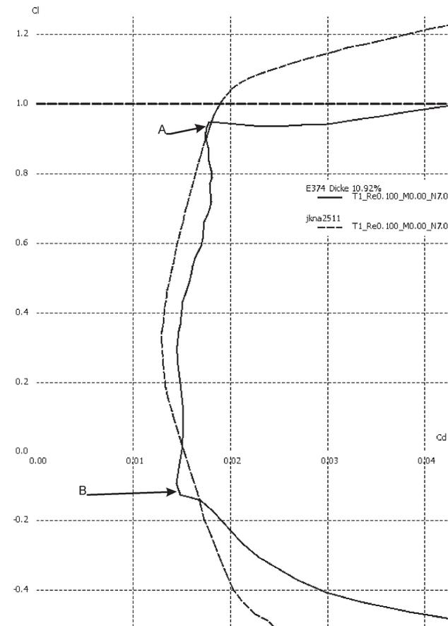
Figure 1. Using an arbitrary value of  $CL$  at low-speed end, e.g. 1.0 (heavy line), would have given an unrealistically poor rating to some foils, as with E374 in this instance. Accordingly I used  $1/L/D_{max}$  for all foils, as measure of high- $CL$  drag. For both foils shown,  $L/D_{max}$  would be near point A. Note how E374 has higher drag everywhere except at two small peaks, A and B.
