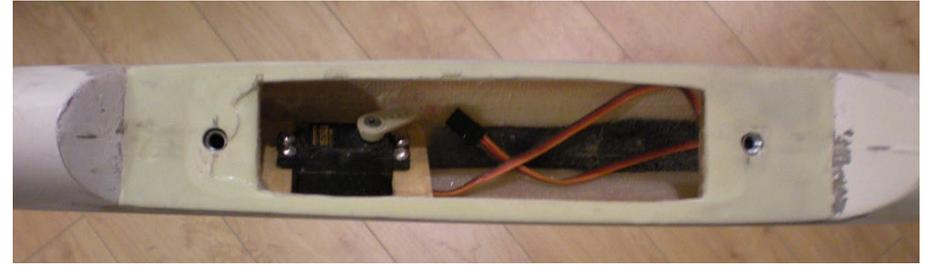
*Left: The wing seat filled in and shaped with the wing.
