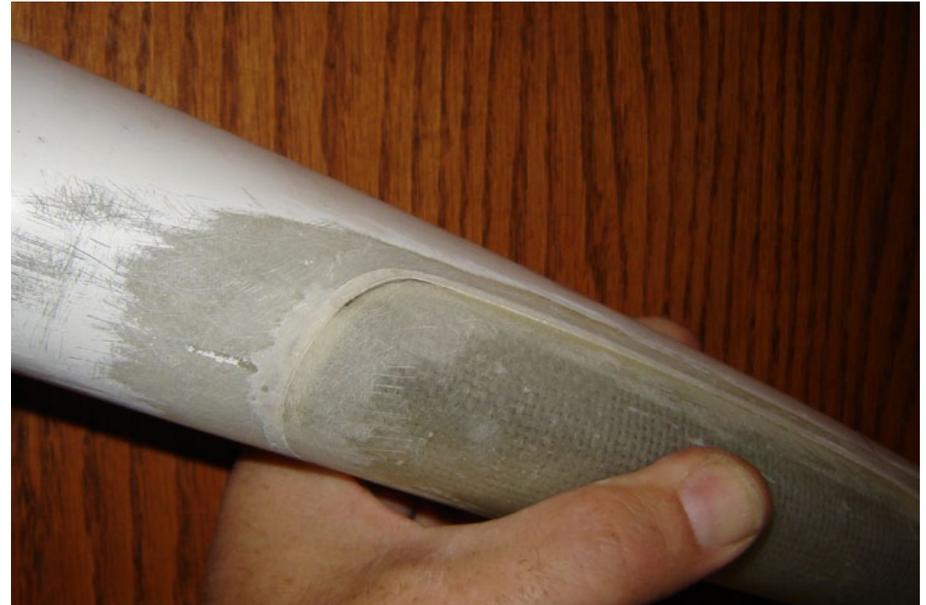
*These photos show the new epoxy added to the fuselage to make a seat for the canopy.*
