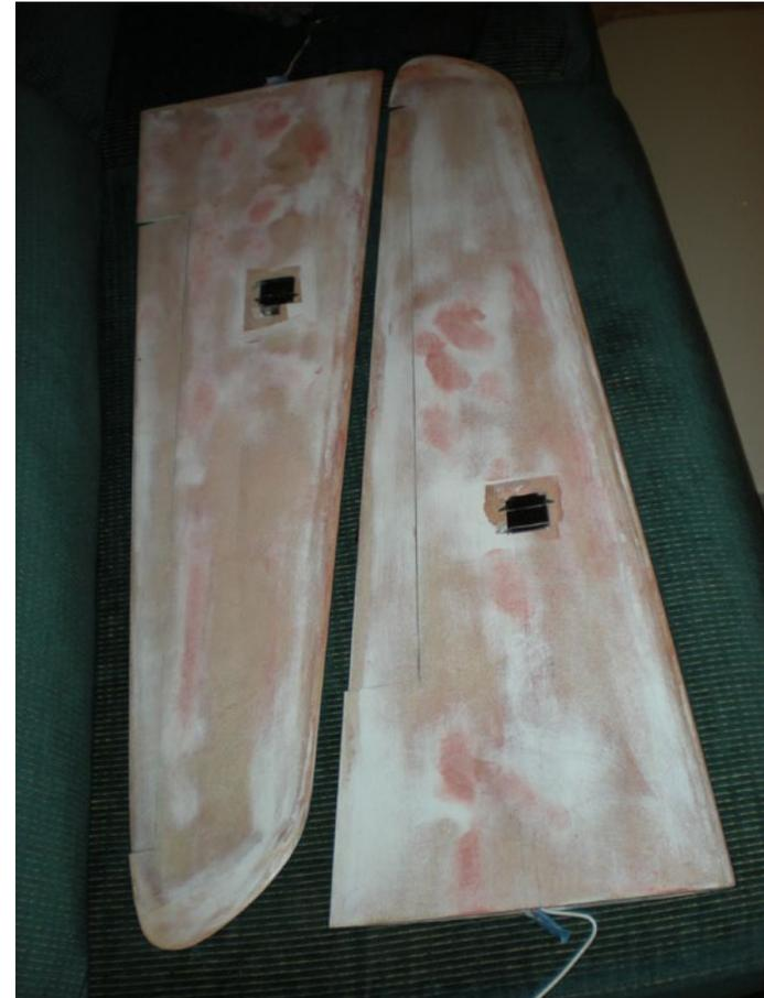
*Right: The servos installed and the ailerons cut out.*
