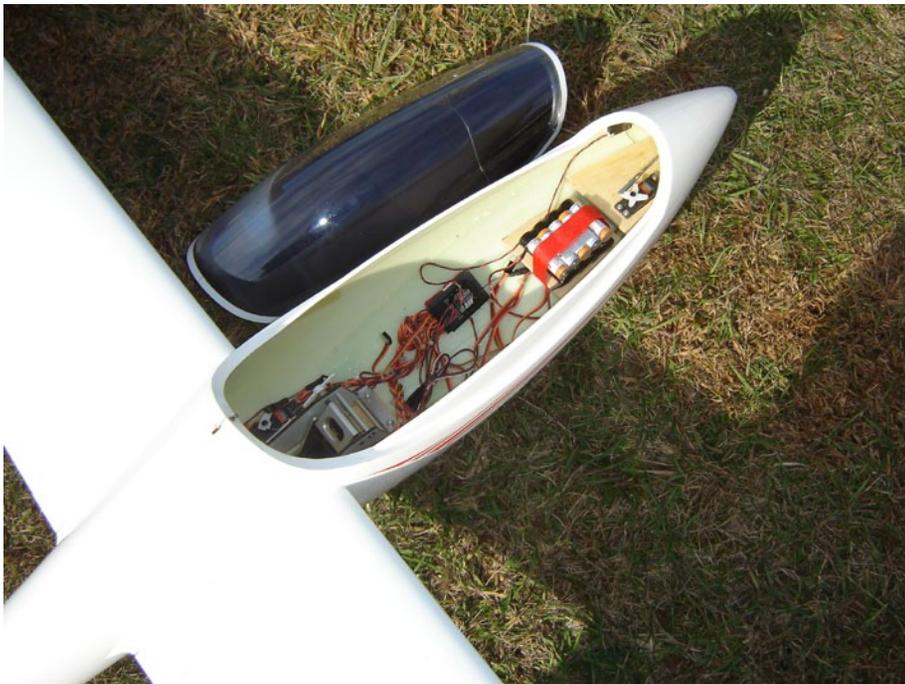
*An excellent example of a radio installation is shown here. The JR receiver is attached with Velcro hook & loop fasteners to the fuselage floor. A 5-cell battery is mounted just aft of the tow-release servo in the nose. The belly wheel is just visible to the rear of the radio room.*
